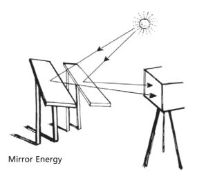
*Solar thermal* systems change sunlight into electricity, by focusing sunlight to boil water to make steam.
